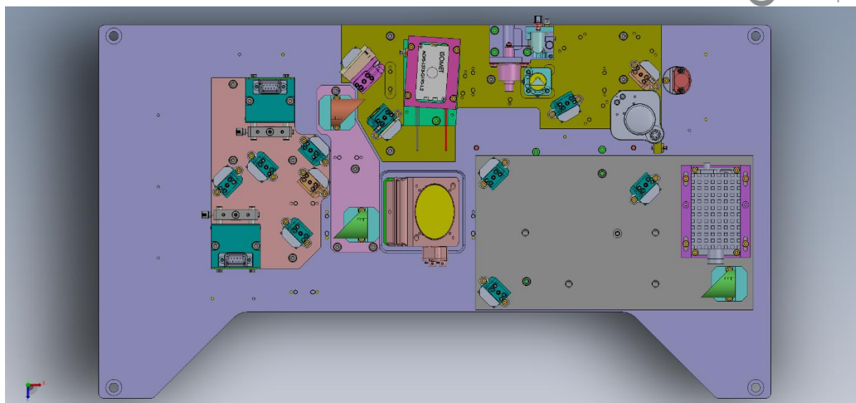
Figure 7: eDrawings representation of the isotope ratiometer designed. The optical system design contains the same optical base (light purple) along with identical laser housing (peach), beam collimation OAP pair (pink), AOM and beam delay (olive) subassemblies. The visual substitutes in a basic sample-detector subassembly (grey). Minor errors or misrepresentations include the presence of the 2-inch gold mirror and mount used for directing the beam out of the original ORION system and the mechanical mirror (silver item between AOM-beam delay and sample-detector subassemblies). Both parts are irrelevant for the isotope ratiometer system, but neither intrudes on the necessary area for modification.
