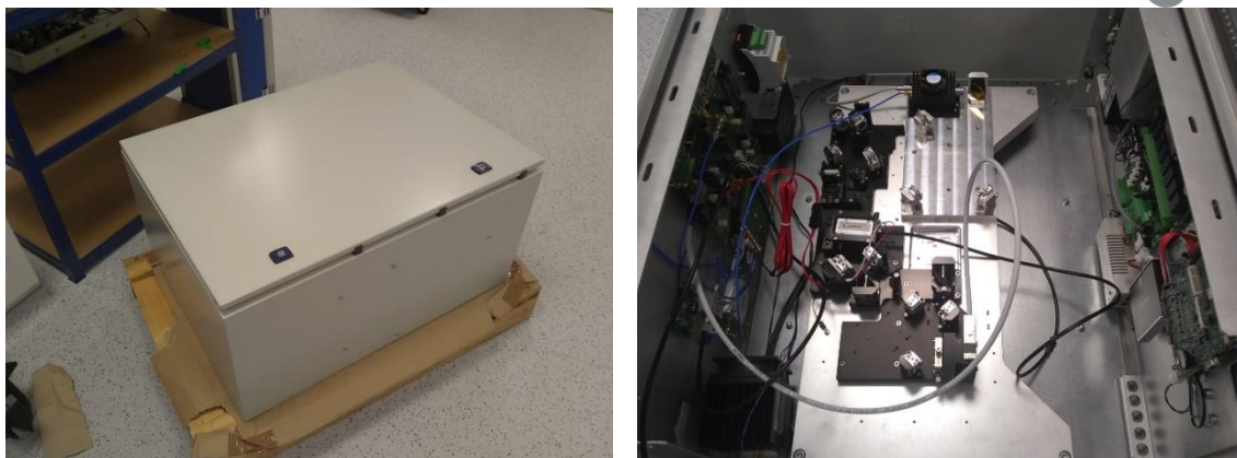
Figure 18: Photographs of the preliminary portable unit. The IP66 case containing the LDS isotope ratiometer (left) can be easily stored in an analogous way that Reykjavik Energy currently does with its electrical switchgear. Inside, the optical base plate, acquisition plate and power supply plate have been successfully mounted. Heat dissipation is primarily controlled by thermal contact between unit plates and the IP66 steel case.
